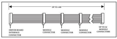
The METRABUS cable used to connect all METRABUS I/O modules to a METRABUS controller is available in standard and non-standard configurations for virtually any arrangement. (See page 550 for ordering details.)
